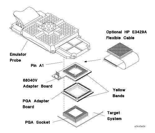
**3** Align pin A1 of your emulator probe with pin A1 on the 68040V adapter board. Attach the emulator probe as shown.
