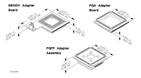
The HP E3440A 68040V Adapter allows the HP 64783A 68040 Emulator, to be used with a 68040V target system. It adapts the 68040V pin-out to that of the 68040V processor and also provides signal and power supply translation from 3.3V to 5V.
