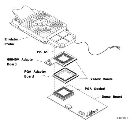
4 Connect the auxiliary power cable from the front of the HP 64700A/B Mainframe to the 68040V Adapter board and then to the demo board as shown below.
